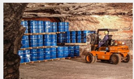
Final disposal of stable HgS in underground facility
