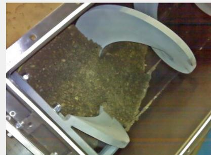
Screw conveyor with dummy material
